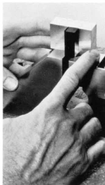
FIG. 4 Jig for Positioning Specimen for Clamping
