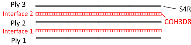
Fig. 6. Layup model schematics of the stacked shell approach.
